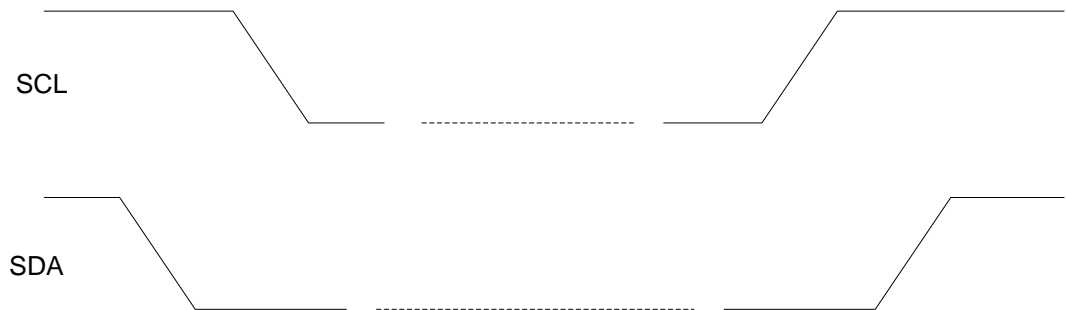
Figure 17: I 2 C START and STOP Condition Timing
