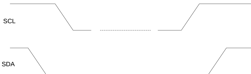
Figure 16: I²C START and STOP Condition Timing
