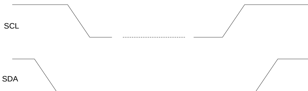
Figure 16: I²C START and STOP Condition Timing
