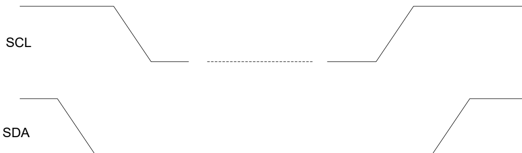
Figure 18: I 2 C START and STOP Condition Timing
