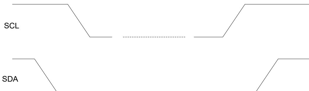
Figure 18: I 2 C START and STOP Condition Timing
