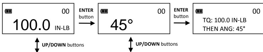
*Note: **UNITS** button can be used to select torque units while on Torque THEN Angle screen.*
