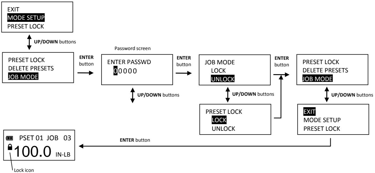
*Note: Text "JOB" is displayed between PSET number and batch count when enabled.*
