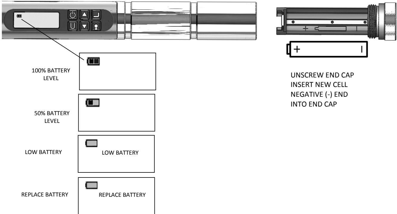
*Note: When Replace Battery screen is displayed wrench will no longer operate until battery is replaced. Only **POWER** button functions which immediately turns off wrench.*
