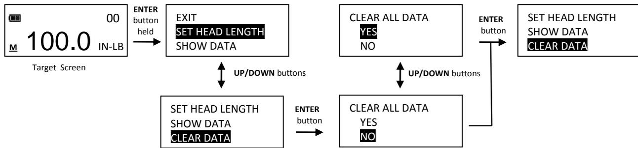
*Note: If wrench is Locked (see Preset Lock in Advanced section), Clear Data function is disabled.*
