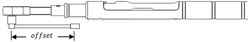
When length of an offset (or sum of head minus offset for interchangeable head) is negative, maximum fastener target is limited by following formulas:
