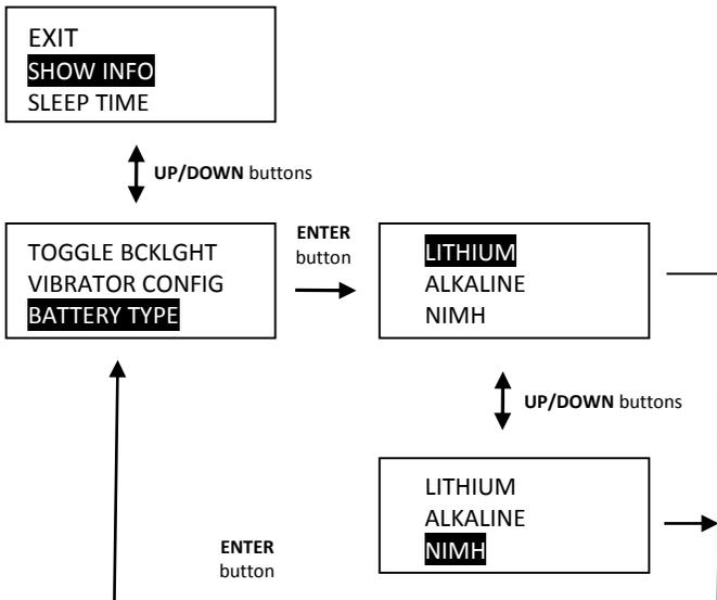
*Note: Wrench is configured for Lithium battery shipped from factory. If Lithium battery is replaced with Alkaline or rechargeable Nickel-Metal Hydride (NIMH), battery type should be changed so battery level icon and LOW battery warnings function optimally. Battery life (REPLACE) will not be impacted, however 50% and Low will be optimized to show most accurate linear discharge time.*
