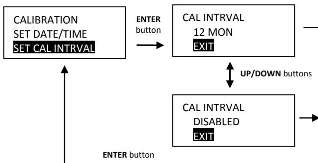
Note: Clock Date and Time must be set before calibration interval will function. If batteries are removed from wrench for longer than 20 minutes, clock will revert to default settings and must be re-entered at power on.
