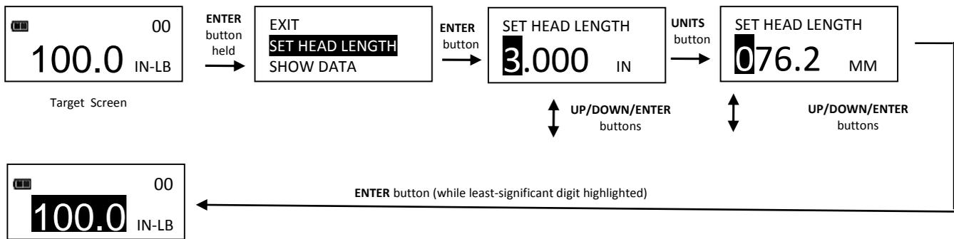
*Note: For a fixed length head, head length entered is offset length measured from center of drive to center of fastener.*
