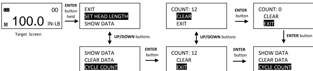
*Note: If wrench is Locked (see Preset Lock in Advanced section) Clear count function is disabled.*
