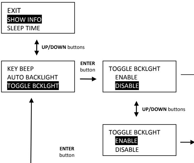
*Note: Backlight will turn off when wrench powers down either by **POWER** button press or sleep time.*
