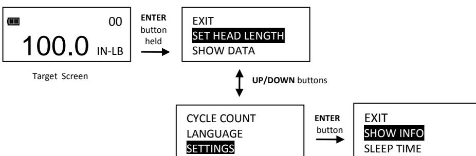
Note: All user configurable settings are stored in non-volatile memory and are retained while power is off.
