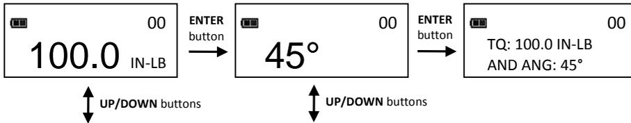
*Note: **UNITS** button can be used to select torque units while on Torque AND Angle screen.*
