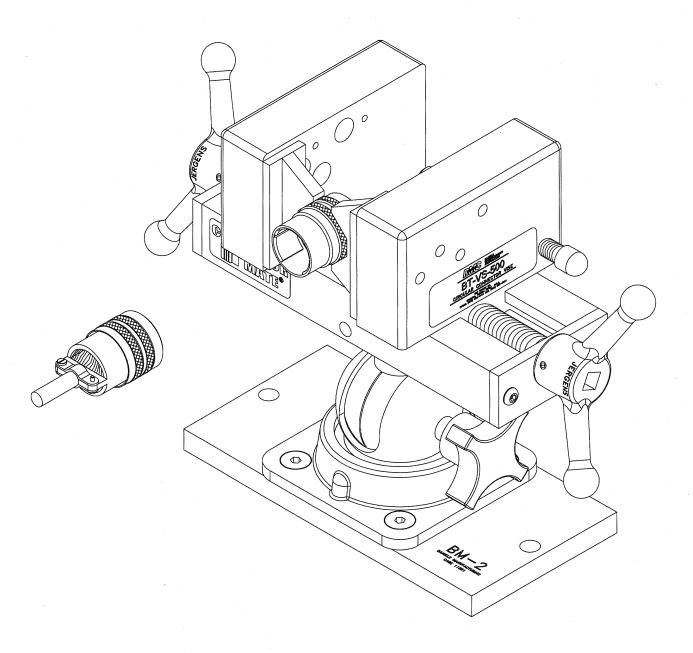
The vise utilizes two complete sets of six (6) different sized pairs of jaw inserts that accommodate diameters from 3/8" to 2", and come in a convenient box. The v-shaped jaw inserts are made of a semi-soft polyurethane material of high frictional characteristics that will not scratch, mar or distort (egg shape) the circular part while securely gripping at  $90^{\circ}$  positions.
