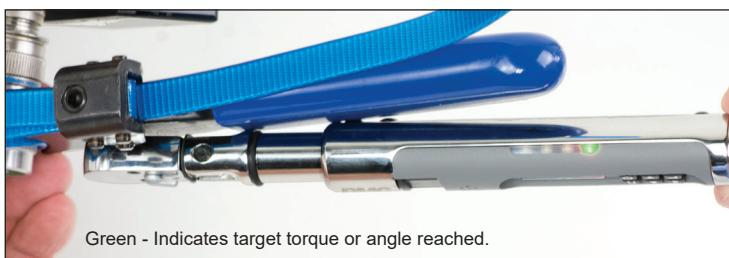
Green - Indicates target torque or angle reached.
