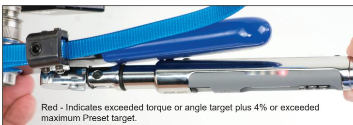
Red - Indicates exceeded torque or angle target plus 4% or exceeded maximum Preset target.
