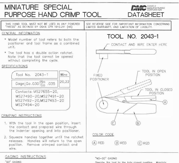
Operate the tool to the fully closed position. Maintain firm hand pressure on the tool handles. Insert the "GO" gage end as shown. The gage must pass freely between the indenter tips. Operate the tool to the fully closed position. Maintain firm hand pressure on the tool handles. Try to insert the "NO-GO" gage end as shown. The "NO-GO" gage may enter the indenter opening, but must not pass completely through the opening.
