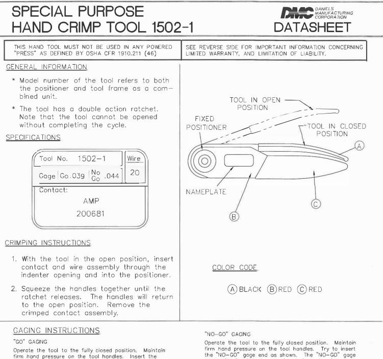
"GO" gage end as shown. The gage must pass freely between the indenter tips.
