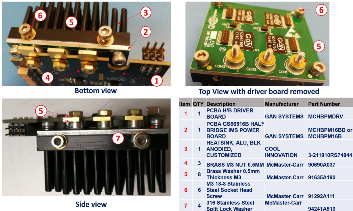
Figure 10 - IMS evaluation module assembly
