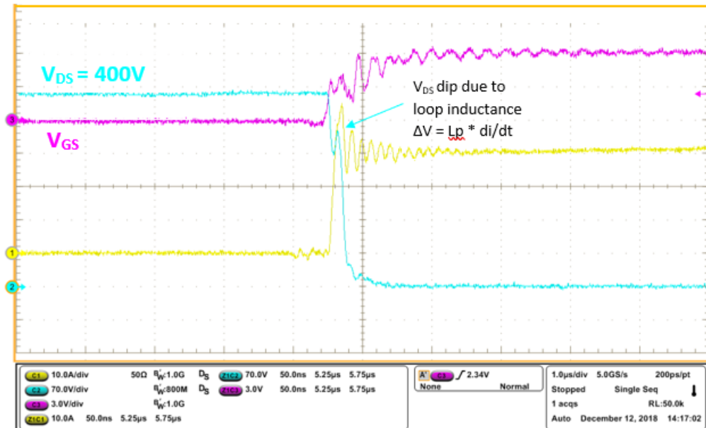
Figure 17 - Double pulse test switching transient - hard switching turn-on 400V/30A
