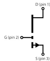
*The thermal pad is internally connected to Source, S (pin 3) and substrate*
