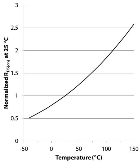
Figure 11: Normalized  $R_{DS(on)}$  as a function of  $T_J$
