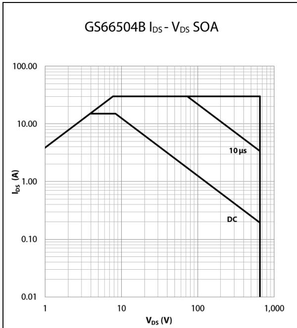
Figure 14: Safe Operating Area @  $T_{case} = 25\text{ }^{\circ}\text{C}$
