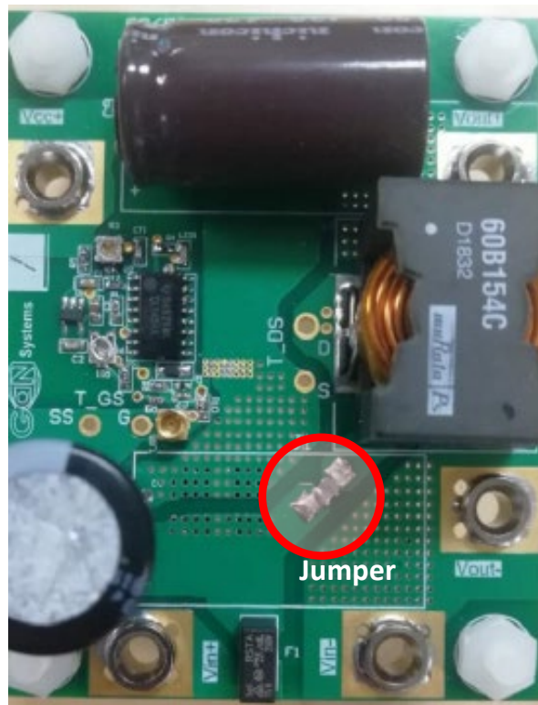
Figure 7 • Current Sensing Jumper Location
