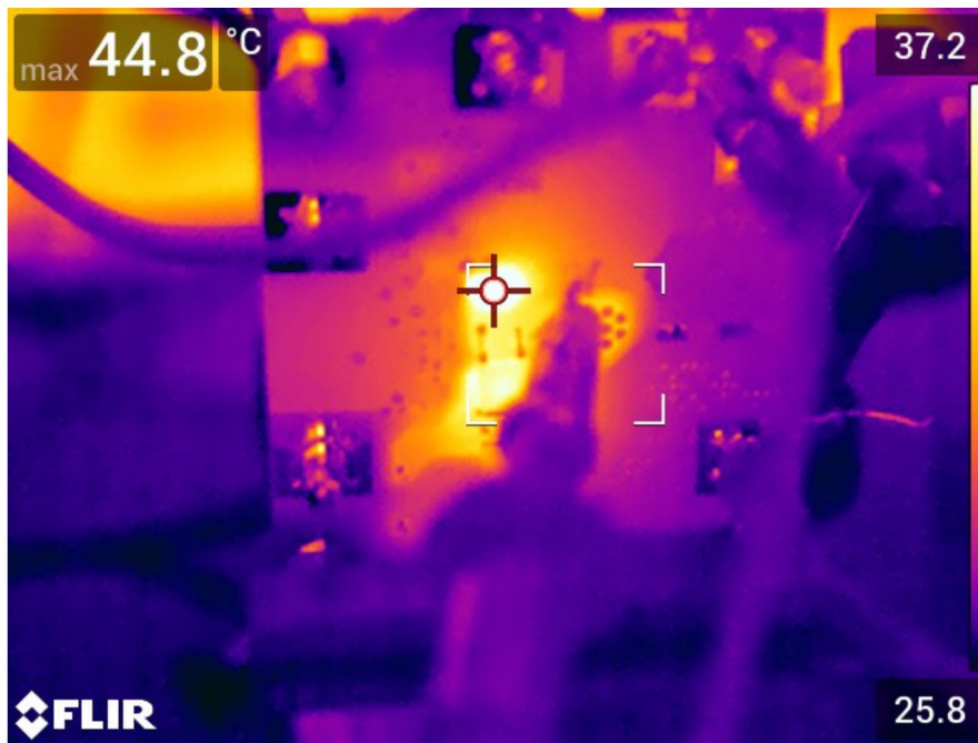
Figure 11 • Thermal imaging with an external fan ( T_{MAX} = 44.8^{\circ}C )
