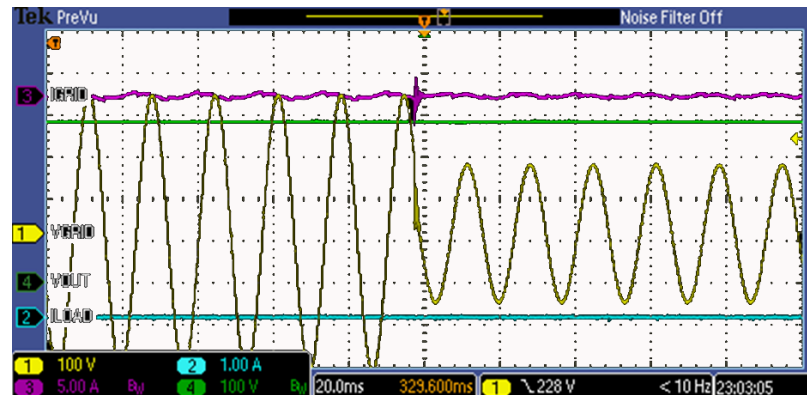
Figure 5.15. AC voltage transient response: from 230 V to 115 V. Ch.1 - V_{Grid} ; Ch.2 - i_{out} ; Ch.3 - i_{Grid} , and Ch.4 - V_{Out}
