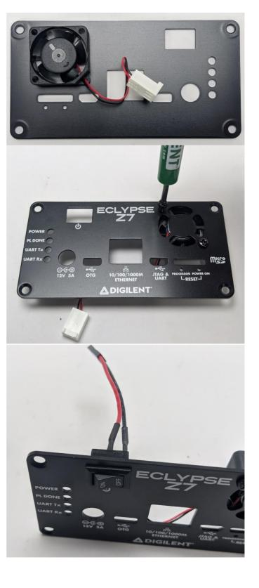
Insert the power switch into the power switch hole and press into place.
