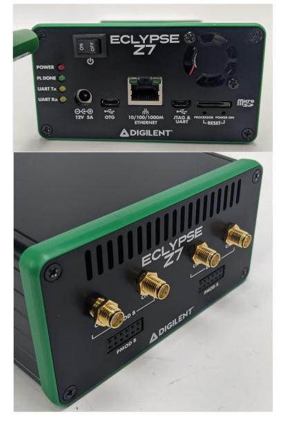
Screw the nuts back onto the SMA connectors.
