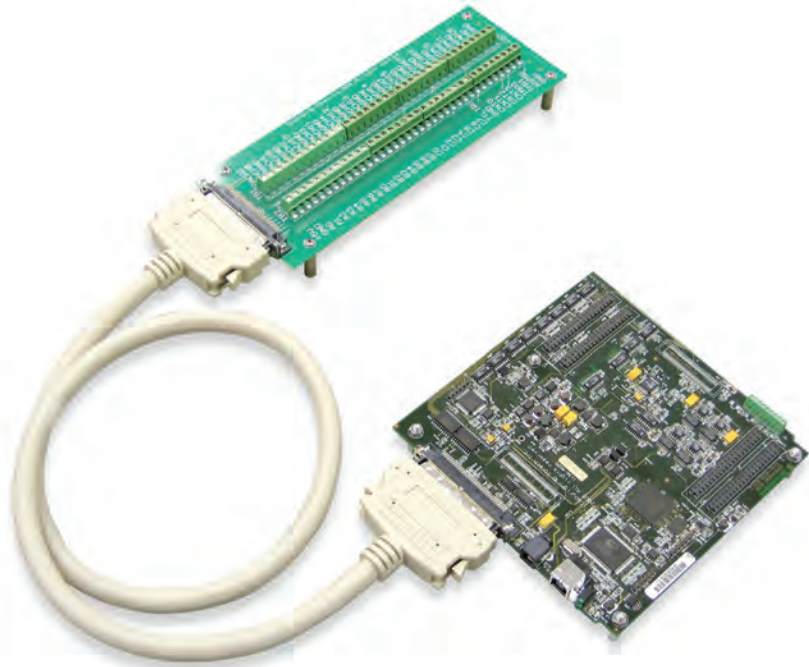
DaqBoard/3001USB attached to a TB-100 screw-terminal board
