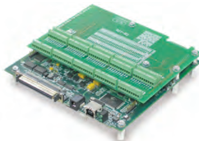
DaqBoard/3001USB with TB-101 screw-terminal board attached
