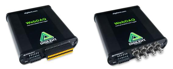
WebDAQ 316: Internet enabled data logger with 16 thermocouple inputs and 4 DIO lines, embedded operating system and web server; includes the ATS018T-W090V power supply with USA, UK, and Europe plugs.
