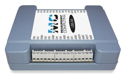
The USB-205 (shown above) provides eight SE analog inputs, two analog outputs, a maximum sample rate of 500 kS/s, 8 digital I/O, and one event counter input.
