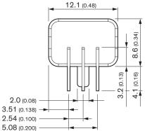
Dimensions in mm (inch) Tolerances:  $x.xx \pm 0.5 (\pm 0.02)$ Tolerances:  $x.xxx \pm 0.25 (\pm 0.01)$ Pin pitch tolerances: ±0.10 (±0.04)
