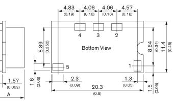
TOS 06-05SM: A = 5.40 (0.21)TOS 06-12SM: A = 6.40 (0.25) Dimensions in mm (inch) Tolerances x.x  $\pm 0.5$  (x.xx  $\pm 0.02$ ) Tolerances x.xx  $\pm 0.25$  (x.xxx  $\pm 0.01$ ) Pin dimension tolerance  $\pm 0.1$  ( $\pm 0.004$ )
