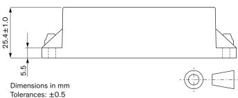
Max. mounting screw tightening torque: 0.29±0.049 Nm (3±0.5 kgfcm)
