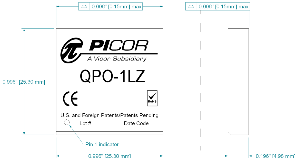
Figure 19 – QPO-1LZ package dimensions.
