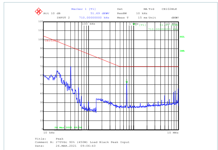
Figure 11 — Peak scan for the BLACK lead, 90% load
