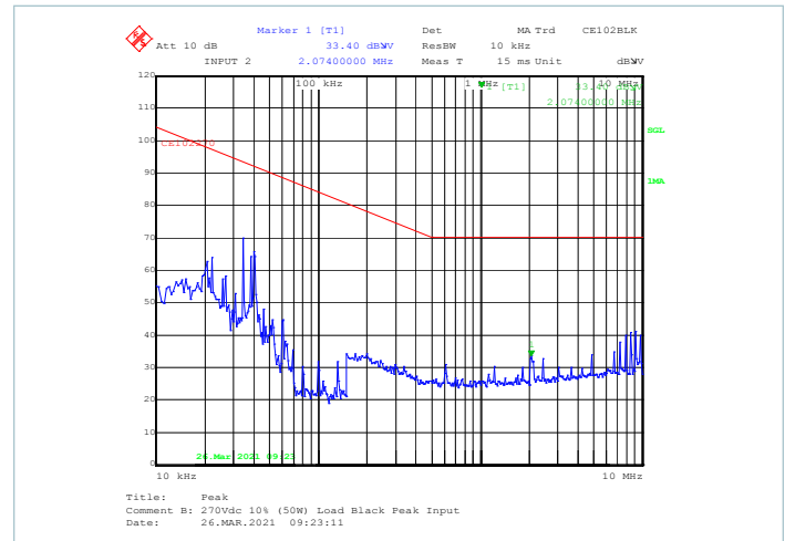
Figure 9 — Peak scan for the BLACK lead, 10% load
