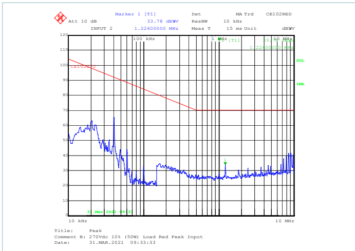
Figure 8 — Peak scan for the RED lead, 10% load
