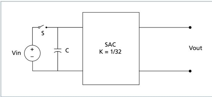
Figure 3 — Sine Amplitude Converter™ with input capacitor
