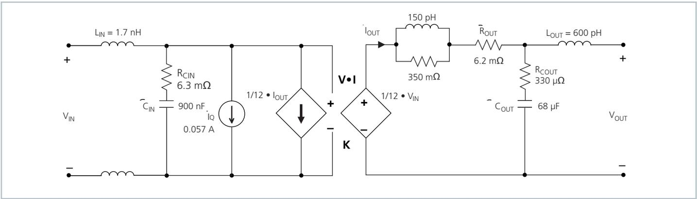
Figure 1 — VI Chip® module AC model (MVTM48EH040M025A00 shown)
