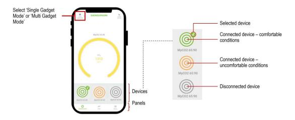
When the gadget logo (concentric circles) is green, it means that the environmental conditions measured by the gadget are deemed comfortable. If a device was connected during the runtime of the application but the connection is subsequently lost, the device logo will appear as grey in the list.
