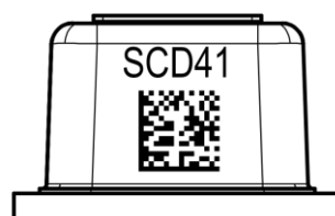
Figure 6: Technical drawing of the laser marking of product type and data matrix on the sidewall of the sensor cap.
