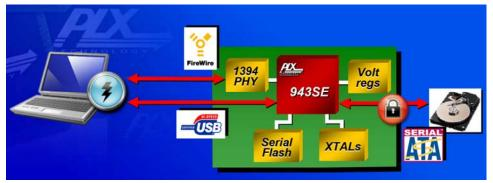
The integrated cipher engine provides advanced encryption and decryption capabilities in hardware and enables OEMs to rapidly deploy full disk encryption solutions, providing end users with peace-of-mind that their private content is safe and secure in the event of theft or loss.
