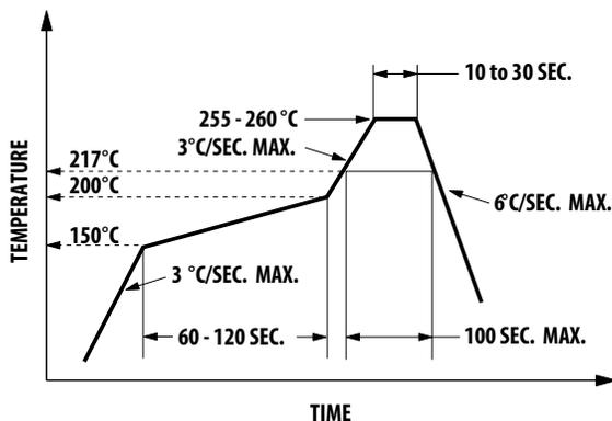
Figure 17 Recommended Board Reflow Direction
