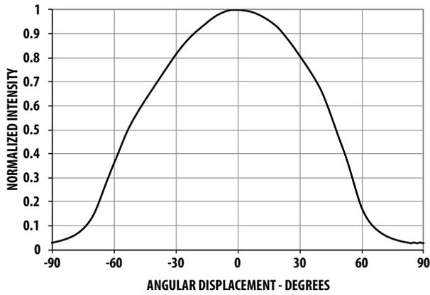
**Figure 8 Radiation Pattern for Minor Axis**
