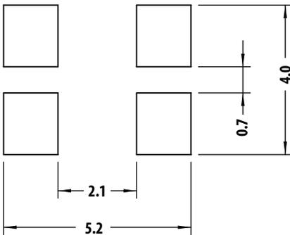
**NOTE** Recommended stencil thickness is 0.1524 mm (6 mils) minimum and above.
