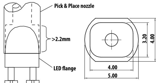
**NOTE** The nozzle tip should touch the LED flange during pick and place.
