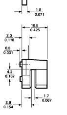
LEAD THICKNESS — 0.25 mm LEAD PITCH — 2.54 mm
