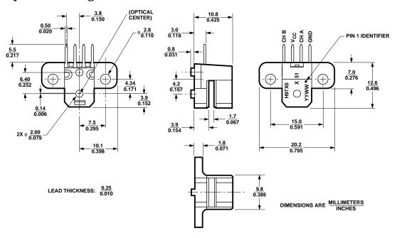
**Mounting Option #51 - Screwmount (Baseplane Mounting)**
