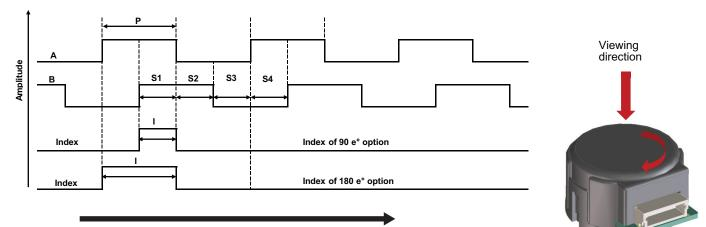
Ch A leads Ch B for clockwise direction, viewed from cover side of the encoder
