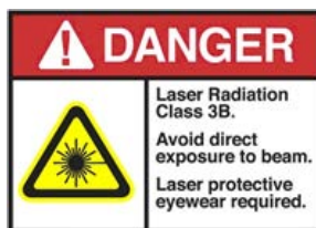
Figure 7: Laser Safety Warning Sign for Unrecommended/Nondefault Operation
