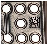
Figure 5: Example Data Matrix Code for Device Identification
