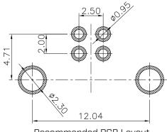
Recommended PCB Layout Top View
