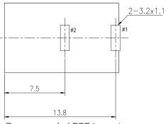
Recommended PCB Layout Top View
