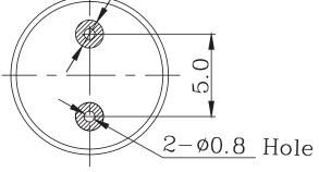
Recommended PCB Layout Top View
