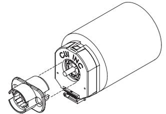
1. Make sure the snaps are fully engaged by pressing on the Hub with the reverse side of Tool C.
