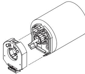
1. Snap the Top Cover onto the Base, carefully observing that the teeth of the Shaft Adaptor align with the grooves in the hub. \*
