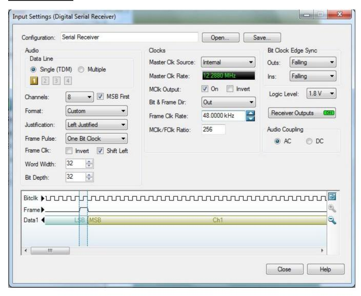
This figure shows an example of a typical timing configuration required to support TDM modes. Please note the SCLK and LRCLK relationship, and edge directions.
