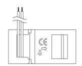
Fan size <40\*40mm, Burr  $\leq$ 0.15mm Fan size 40\*40 $\sim$ 80\*80mm, Burr  $\leq$ 0.25mm Fan size >80\*80, Burr  $\leq$ 0.3mm
