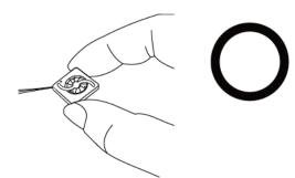
Don't pull fan with lead wires.
