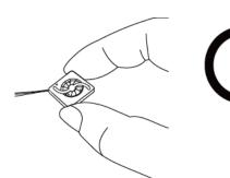
Don't pull fan with lead wires.
