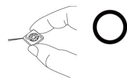
Don't pull fan with lead wires.
