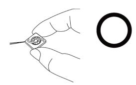
Don't pull fan with lead wires.
