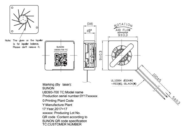
Sunon standard sample exclude the connector. If there is any request for connector, please advise in advance. About recommend connector, SUNON recommend the following models for SUNON Mighty Mini Fon/Blower: 1.(JST) SUR series connector: 02SUR-32S / 03SUR-32S / 04SUR-32S.
