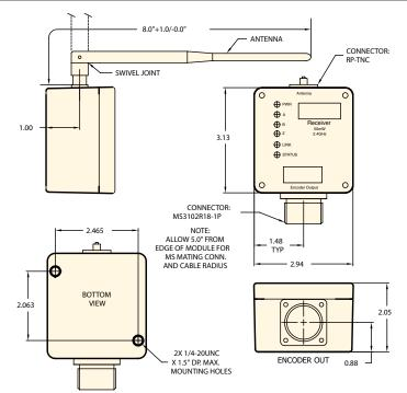
The SwiftComm Receiver Module has an MS connector that provides the same output signals as a standard BEI encoder. Input power can be from 5 to 28 VDC. Quadrature output signals (specified at time of ordering)
