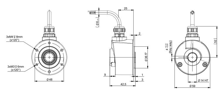
Note: A key (4x4x8) ensuring the positive locks function between driving shaft and encoder is provided in the encoder box.
