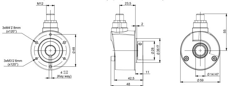
Note: A key (4x4x8) ensuring the positive locks function between driving shaft and encoder is provided in the encoder box.
