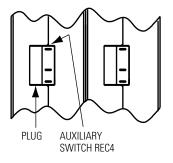
Alarm & Auxiliary Switch Combination
