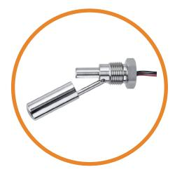
The TSSF212 series is a compact external fitting device, via 1/2"NPT thread, with a high specification thermistor so capable of sensing both liquid level and temperature.
