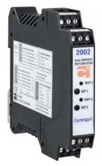
The SC2002ALM-HL trip amplifier can accept a wide range of user configurable inputs including 4-20mA, 0-20mA, 0-5V and 0-10V. The unit can have up to two relay outputs and each can operate as a high or a low trip: alternatively latching operation using both trip points can be configured.
