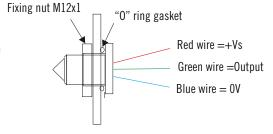
Note. LLPK1 - Nitrile 'O' ring and Nickel plated brass M12 nut kit - is available as an optional extra.
